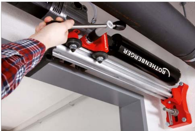
Dowel plate: Extremely small dimensions, for very tight spaces
