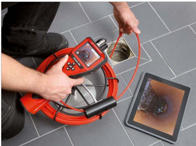
Inspection of basin drains
